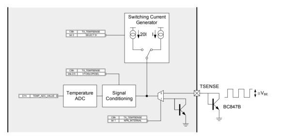
Figure 17 – Temperature sensor functional block diagram
