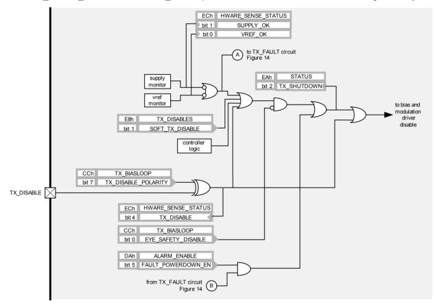
Figure 16 - Transmit Shutdown Generation
