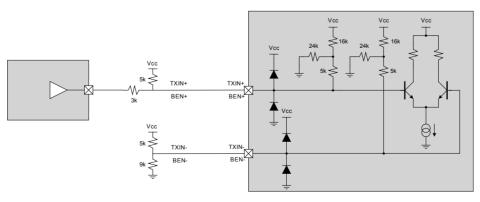
Figure 36 – Single-ended CMOS/LVTTL interface for BEN
