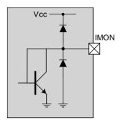
Figure 29 - MPD input structure
