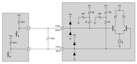
Figure 34 - DC-Coupled CML interface for TXIN and BEN
