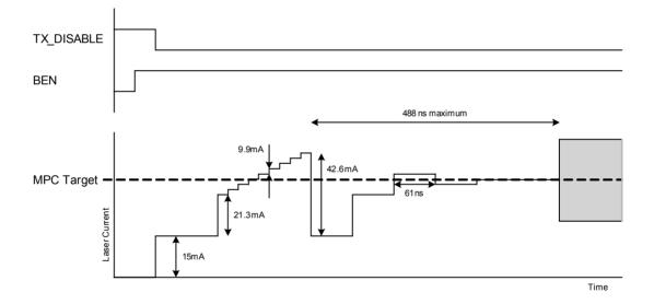
Figure 39 - Closed Loop Fast Start-up Algorithm Example
