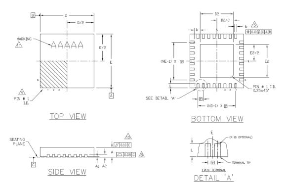
Figure 40 – 32pin TQFN Package Dimensions
