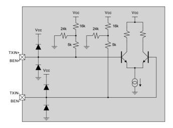
Figure 25 - Transmit input structure
