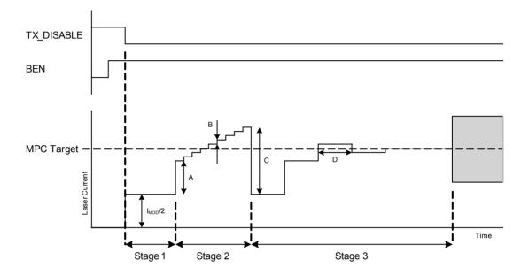
Figure 38 - Closed Loop Fast Start-up Algorithm
