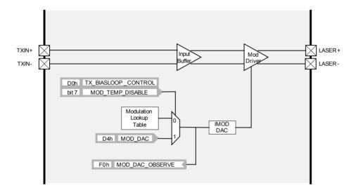
Figure 11 - Modulation Current Generation
