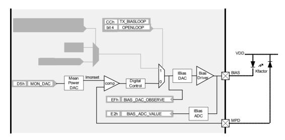
Figure 14 - Bias Current Generation, Closed Loop
