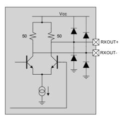
Figure 28 - Receive output structure
