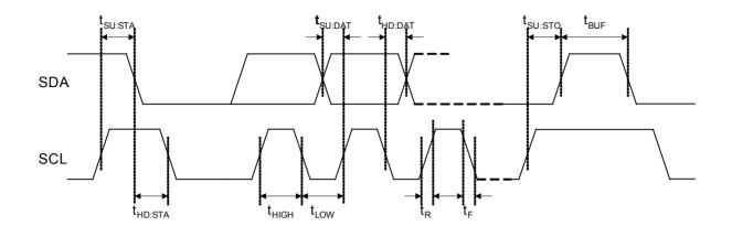
Figure 8 - SDA and SCL bus timing
