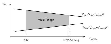
Figure 4 – Valid combinations of transmitter input voltages
