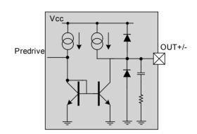
Figure 26 - Transmit output structure
