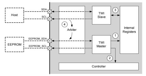
Figure 18 - Serial interfaces to internal registers
