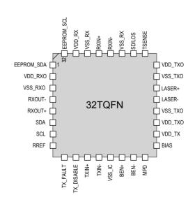
Figure 2 – Device pin out
