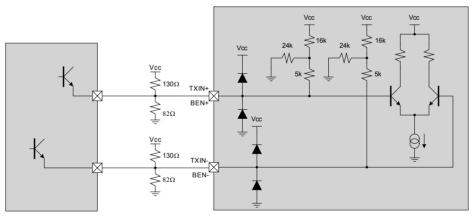
Figure 35 - DC-Coupled LVPECL interface for TXIN and BEN
