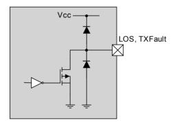
Figure 31 - LOS/TX\_FAULT output
