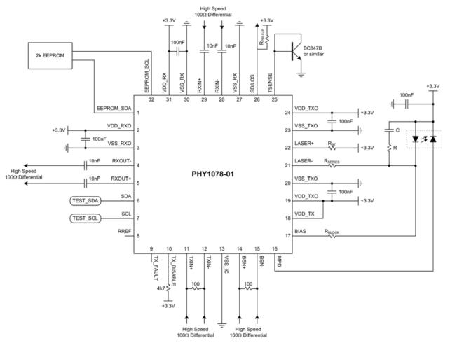
Figure 32 – Typical ONU Application Diagram
