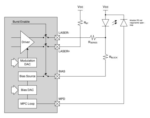
Figure 37 - DC-Coupled Laser Application Diagram
