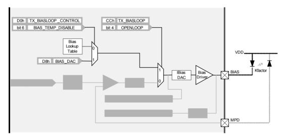
Figure 13 - Bias Current Generation, Open Loop
