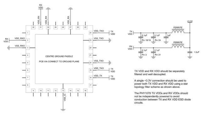
Figure 33 – Recommended power supply connections and filtering.
