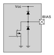
Figure 30 - Laser bias output structure
