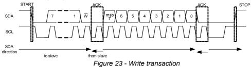
If the slave is unable to receive data then it should return a NACK after the data byte. This will cause the master to issue a STOP and thus terminate the transaction.
