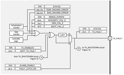
Figure 15 - Transmit Fault Generation
